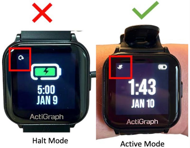
10. Confirm that the watch displays a “running” icon in the top left corner. This indicates that the device is in *Active mode* and has begun collecting data.
