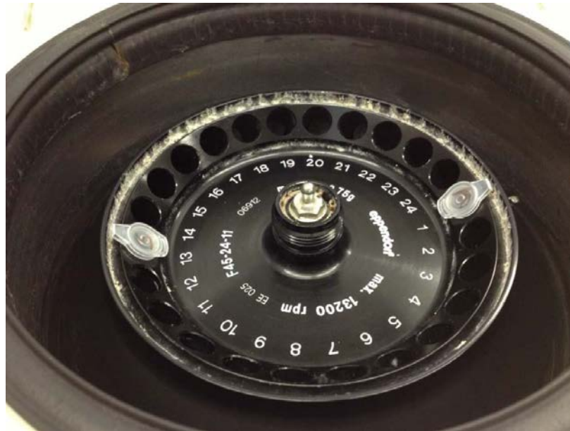
Figure 8: Example of centrifuge tube counterbalancing placement
