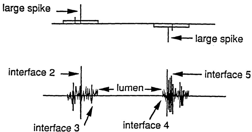
Figure 13. Ideal Image of Artery on Channel 2 of Oscilloscope Screen
