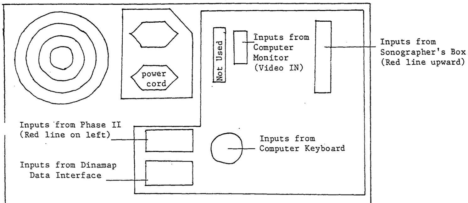
Figure 4. Ultrasound Assessment Equipment: Computer - PC 486
