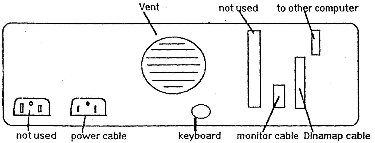
Figure 6. Ultrasound Assessment Equipment: Computer IBM-XT
