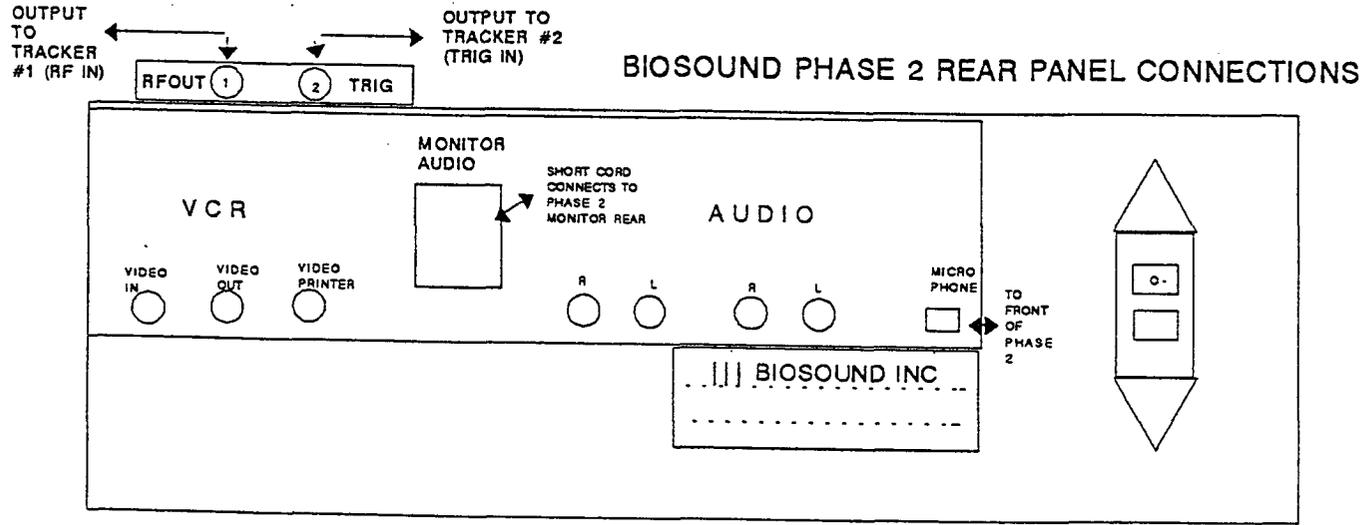
Figure 1. Ultrasound Assessment Equipment: Biosound Phase 2 VCR
