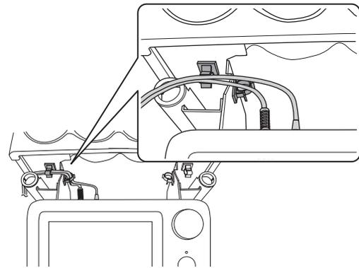
4. Disconnect the ECG clip and the PCG sensor from the connectors on the back of the main unit.
