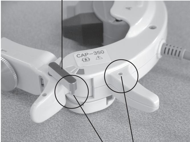
The projecting part of this lever is inserted into this hole.
