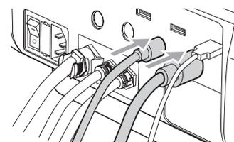
**14.** Secure the ECG clip and the PCG sensor cables in the cable notch and fasten the two cable fasteners.
