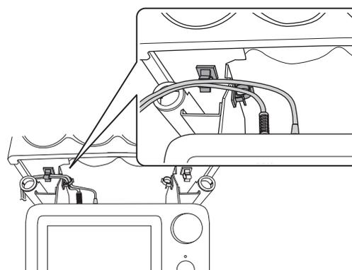
4. Disconnect the ECG clip and the PCG sensor from the connectors on the back of the main unit.
