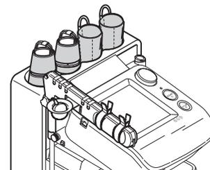
5. Hang the sensor box cable on the cable hook.
