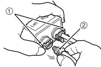
2. Insert each connector on the new cuff into the sensor box until it clicks into place.
