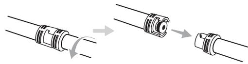
2. Insert the connector on the new cuff into the air hose. Rotate the connector clockwise until it clicks into place.
