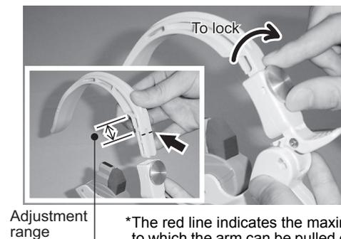
\*The red line indicates the maximum point to which the arm can be pulled out. Do not pull the arm out beyond this line.
