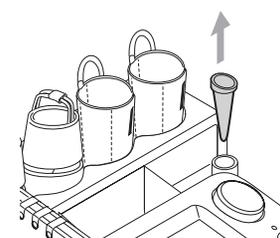
6. Loosen the screw ① and pull out the arm.
