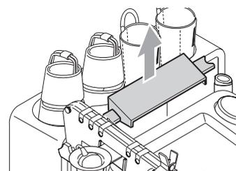
3. Detach the cables (one for the ECG clips and the other for the PCG sensor) from the fasteners behind the main unit.
