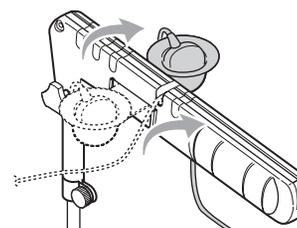
11. Attach the arm rail and PCG sensor cable fastener ⑤, and tighten screw ④.
