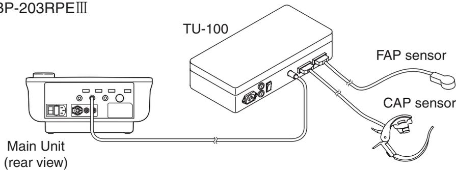
**Caution** Please be sure to turn off the main unit power before removing or connecting each unit and sensors. Otherwise electric shock or device failure may result.
