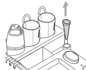
6. Loosen the screw ① and pull out the arm.
