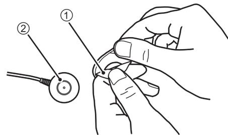
**3. Remove the clear protective sheet from the PCG sensor pad ③.**
