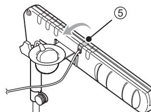
10. Move the PCG sensor cable and the PCG sensor pocket to the outer side.
