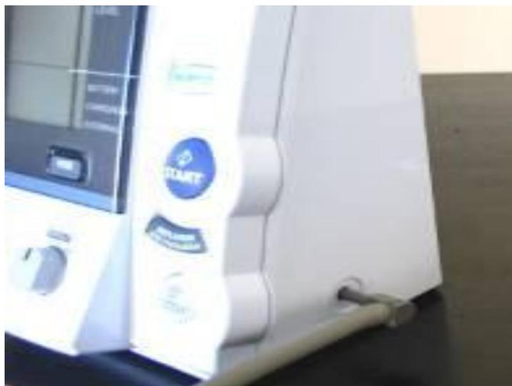
For all cuff sizes small, medium, large, and X-Large connect the air tube to the main unit by attaching the air plug to the base of the air connector. Connect the cuff to the air tube attached to OMRON unit Wrap and secure the appropriate cuff to the participant's upper right arm as set out in section 13.2.7, above.
