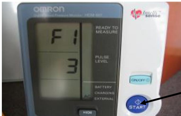
Push the START button and F2 function is displayed in the first window and 0 waiting time is displayed in the middle window (Figure 13.7)
