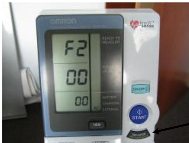
If needed push the DEFLATION (deflation control)/Measurement Result Display Switch Button and change the set value to 0 sec waiting time. Push the START button and F3 function is displayed in the first window and inflation interval 30 second time is displayed in the bottom window (Figure 13.8).
