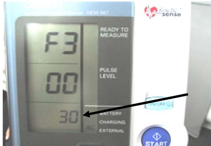
If needed push the DEFLATION (deflation control)/Measurement Result Display Switch Button and change the set value to 30 sec measurement interval.
