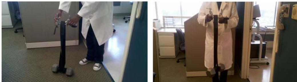
Average the three calibration trials. The dynamometer should be accurate within  $\pm 2$  kgs for the average of the three calibration trials. If the result is outside the  $\pm 2$  kg range after following the Troubleshooting tips below, you must send the dynamometer to the manufacturer for repair and recalibration. **DO NOT attempt to recalibrate the dynamometer yourself.** Calibration problems can be caused by dropping the dynamometer or by leaks in the hydraulic system.
