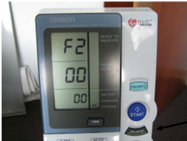
If needed push the DEFLATION (deflation control)/Measurement Result Display Switch Button and change the set value to 0 sec waiting time. Push the START button and F3 function is displayed in the first window and inflation interval 30 second time is displayed in the bottom window (Figure 10.8).
