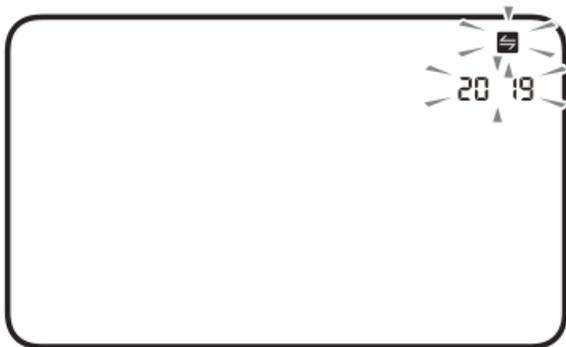
Press the Bluetooth button on the back of the monitor to change the year. If the correct year is already displayed, skip this step.
