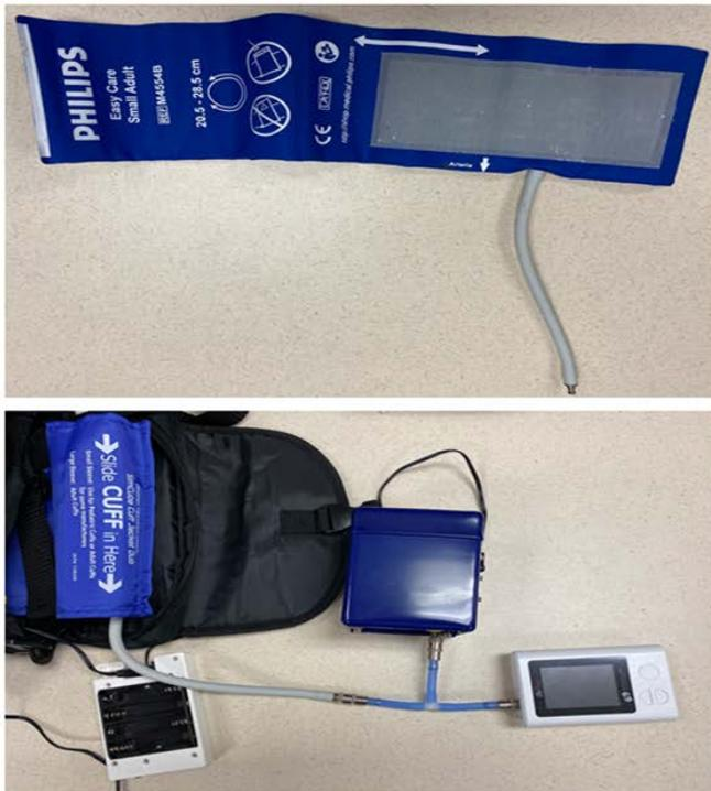
Insert the cuff (small cuff size) into the cuff sleeve. Connect the ABPM device to the simulator and the cuff using the appropriate adapter. Plug the SimCube power supply into an AC outlet
