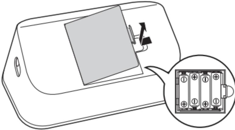
Close the battery cover. Consider taping the back of the device to prevent batteries coming out if the monitor is dropped.
