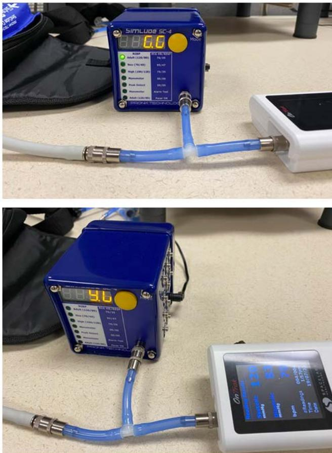
The LED on the simulator should read 0.0 before you start the reading. Push the action button and wait for the reading to complete.
