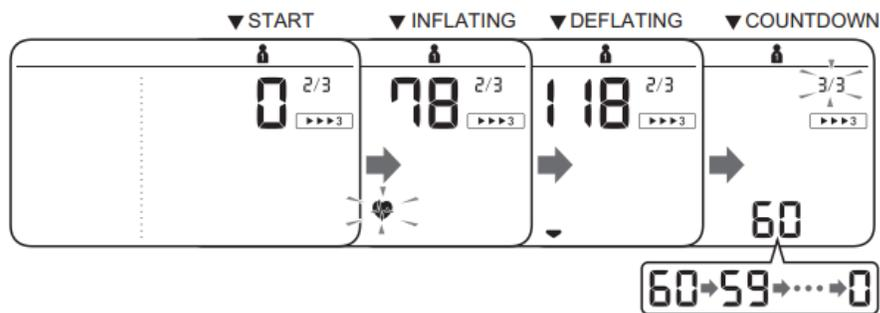
After the third measurement is complete, the average for the 3 measurements appears on the display.
