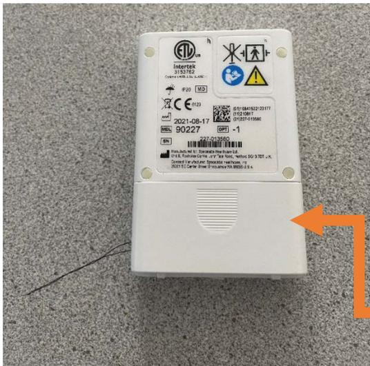
The back cover can be secured over the piece of string or ribbon.
