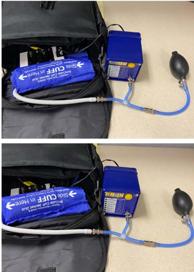
The LED on the simulator should read 0.0 before you begin to manually pump the bulb. You should expect an increase in size of the cuff with every pump of the bulb. When you reach 150mmHg on the simulator, observe for a gradual decrement in the mmHg.
